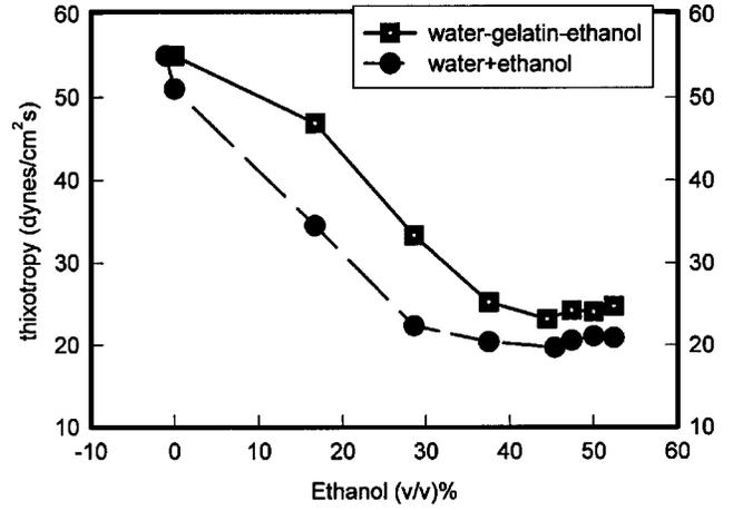
FIG. 9. Variation of the solution thixotropy as a function of the ethanol concentration for aqueous solutions with the without gelatin. Notice that the presence of ethanol increases the solution thixotropy significantly.
