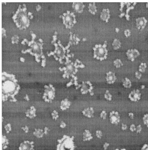
FIG. 5. Scanning probe micrograph ( $10 \times 10 \mu\text{m}^2$ ) of the same sample as in Fig. 3(a) after seven days. Notice the popcorn shaped aggregates, which typically have 500-nm aggregates at the core. The corona has a fractal dimension  $d_f = 1.59 \pm 0.5$ .
