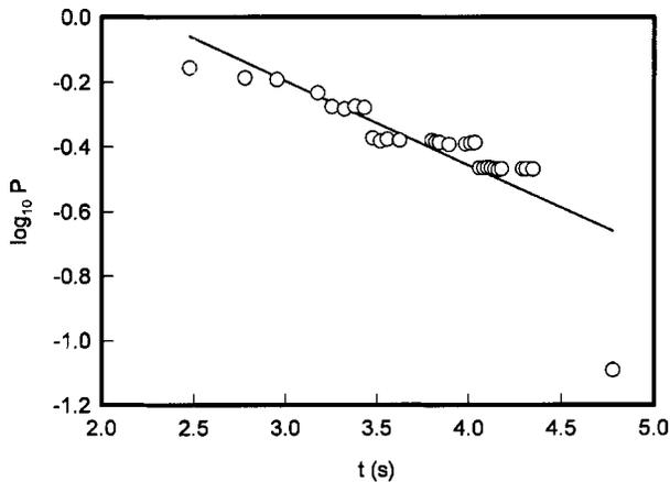
FIG. 8. Temporal variation of the polydispersity parameter  $P$  of aggregated gelatin molecules in aqueous solutions measured by dynamic light scattering. The data fitting yielded  $P \sim t^{-0.2}$ .
