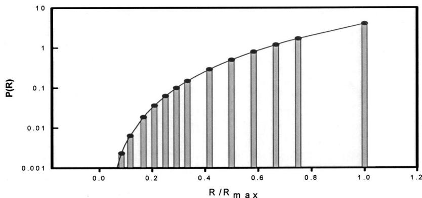
FIG. 2. Dynamic light scattering measurement of the particle size distribution of the same sample as in Fig. 1. Fitting to Eq. (1) gives  $\alpha=4.01$ .
