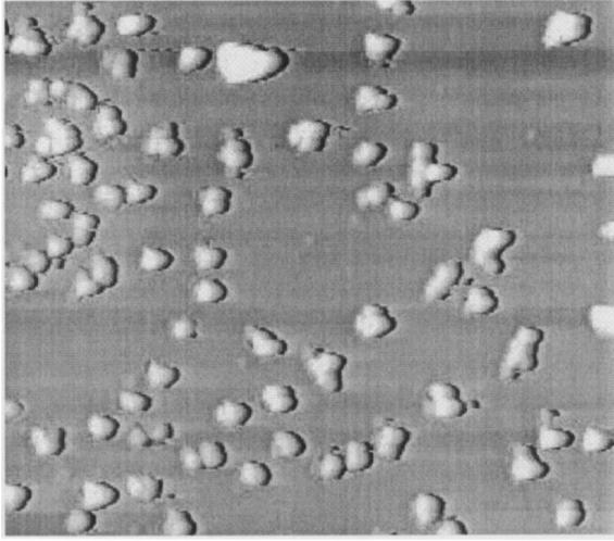
FIG. 6. Scanning probe micrograph ( $10 \times 10 \mu\text{m}^2$ ) of the same sample as in Fig. 3(a) after 14 days. Notice that the popcorn shaped aggregates seen earlier in Fig. 5 have melted to give rise to typically 500-nm aggregates all over.
