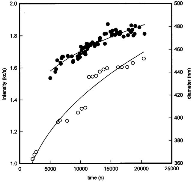
FIG. 7. Temporal growth of effective diameter  $R_h(t)$  (○) and intensity (●) of light  $I_s(t)$  scattered from aggregated gelatin molecules in aqueous solutions measured by dynamic light scattering. The data fitting to  $R_h(t) \sim I_s(t) \sim t^{1/d_f}$  gave  $d_f = 2.6 \pm 0.2$ .
