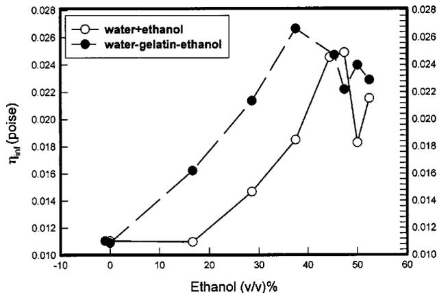
FIG. 10. Variation of the solution viscosity at infinite frequency as a function of the ethanol concentration for aqueous solutions with and without gelatin. Notice that the presence of ethanol increases the solution thixotropy significantly, and close to an ethanol concentration of  $\approx 45 \pm 2\%$  v/v there is a dip in the viscosity value. This is the region where fractal aggregates are formed on hydrophilic substrates.
