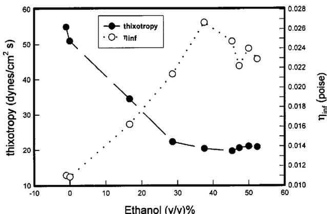
FIG. 11. Comparison of the solution viscosity at an infinite frequency as a function of the ethanol concentration for aqueous gelatin solutions. Notice that the solution thixotropy rises close to an ethanol concentration of  $\approx 45 \pm 2\%$  v/v, where there is a dip in the viscosity value. This is the region where fractal aggregates are formed on hydrophilic substrates.
