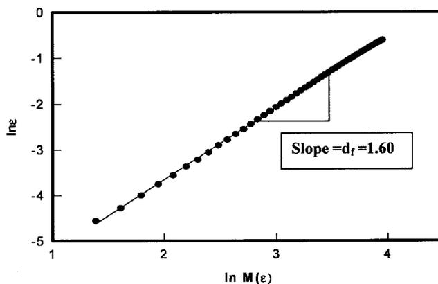
FIG. 4. Double-logarithmic plot of  $N(\epsilon)$  vs  $1/\epsilon$  for the gelatin aggregates shown in Fig. 3(a) for the aggregates formed on glass substrate. The fractal dimension is deduced from the slope.
