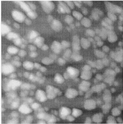
FIG. 1. Scanning probe micrograph ( $5 \times 5 \mu\text{m}^2$ ) of a 1%  $w/v$  aqueous gelatin solution with 0.1M NaCl taken at 25 °C in the tapping mode. The picture shows gelatin aggregates of sizes 65 nm, 190 nm, 380 nm, and larger clusters. Tiny particles seen in the background are single molecules of typical size 30 nm.
